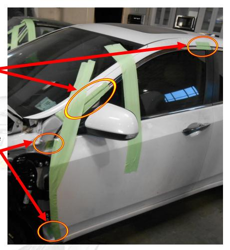
After marking the door and disconnecting the wire harness remove the door factory hinges.
