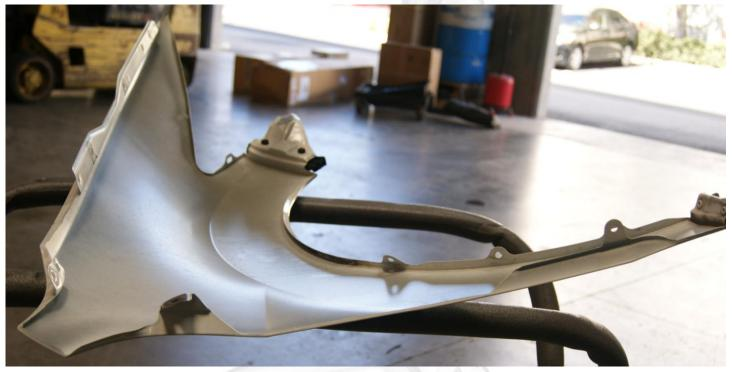
Close the door and replace the fender by reversing step 2.
