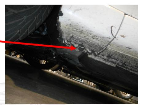
Open the door and remove the bolt securing the fender to the body by the top factory door hinge as shown '
