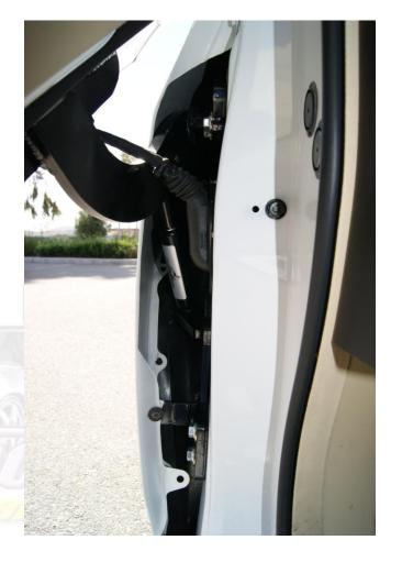
Cut the inner lip of your fender to make room for the new Vertical Doors hinge. Note: After you have cut the fender use a sander or grinder and make sure the surface is completely flat.
