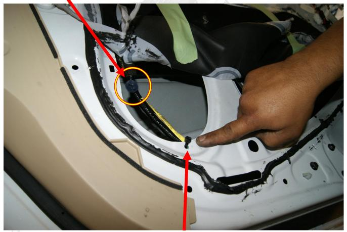
Used zip ties to secure the wire to the door as shown.
