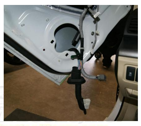
door wire harness. Use zip ties to secure the wires back to the door once you gain the extra wire harness.
