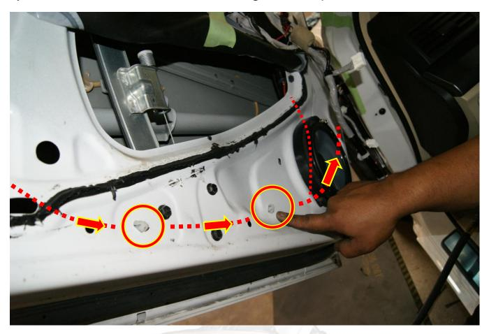
Once you have gained the necessary wire slack you can replace the door panel.
