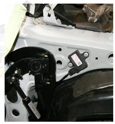
Page 5 of 12 Acura TSX 08-14 You will need extra wire slack to allow the VDI hinge system to work properly.
